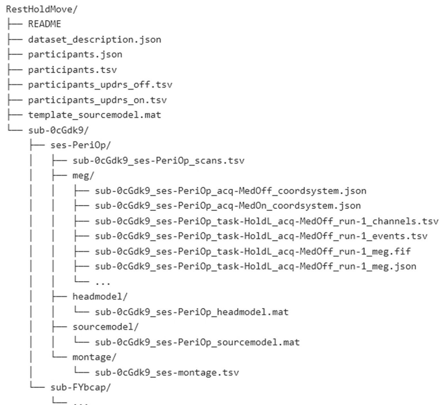
Fig. 3 Dataset structure. Brain Imaging Data Structure (BIDS) showcasing the hierarchical arrangement of files.
